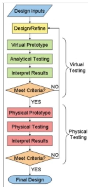
Fig. 24-1. Engineering design process for complex systems
