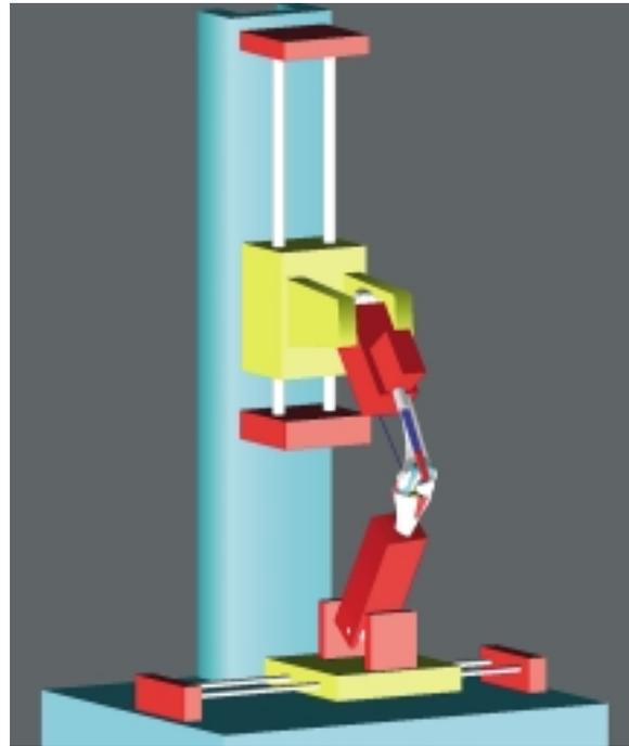
■ Fig. 24-2. The Virtual Knee simulates lower leg in vivo functional activities for the purpose of evaluating the kinematic and kinetic performance of TKR designs
