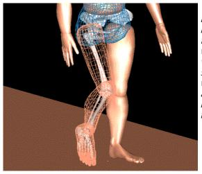
Walk this way: Using leg and foot measurements plus the patient's age and weight, a customized version of ADAMS simulates his gait, with limbs displayed as realistic solid models or in skeletal form.
